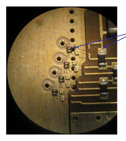
Switches and the control circuitry are integrated into a thin IC
